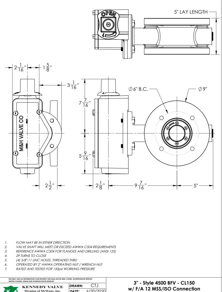
KENNEDY VAL Division of McWane, In 1021 East Water St. Elmira, NY 14901 DRAWN: C13 DATE: 6/30/2020 DWG: NO. BD03-F1-M11-000 3" - Style 4500 BFV - CL150 w/ F/A 12 MSS/ISO Connection BURIED OPERATOR - OPEN LEFT FLANGED ENDS
