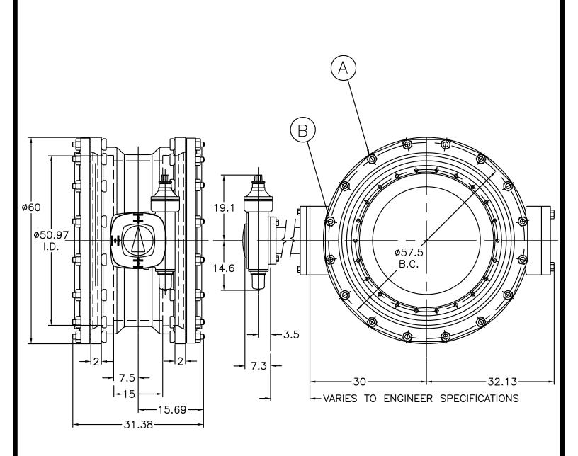
NOTE 2: VALVE SHAFT WILL MEET OR EXCEED REQUIREMENTS OF SHAFT TABLE PER AWWA STANDARD C-504 FOR APPLICABLE CLASS.
