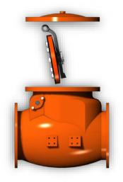
b.Allow a minimum of one pipe diameter on one side of the valve and 2.5 diameters on the opposite side for the removal of the hinge pin (see picture below).
