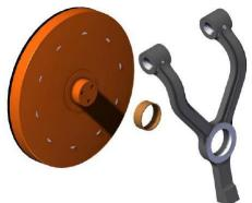
10. Remove the **BOLTS** and **WASHERS** holding the **ENCAPSULATED RESILIENT SEAT RING** on to the **CLAPPER DISC**, and then remove the **ENCAPSULATED RESILIENT SEAT RING**.
