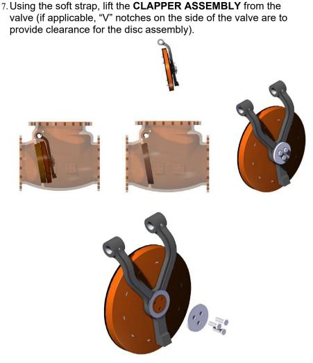
8. Remove **CLAMP PLATE BOLTS**, and **CLAMP PLATE** from the
