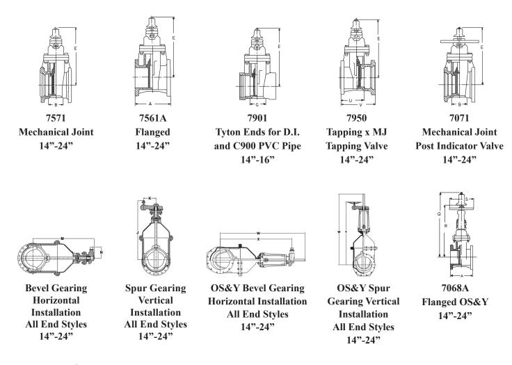
**NOTE:** It is recommended that valves be installed with stems vertical when used in raw sewage or sludge applications or in water with excessive sediment. Flanged end connections not recommended for burial service.
