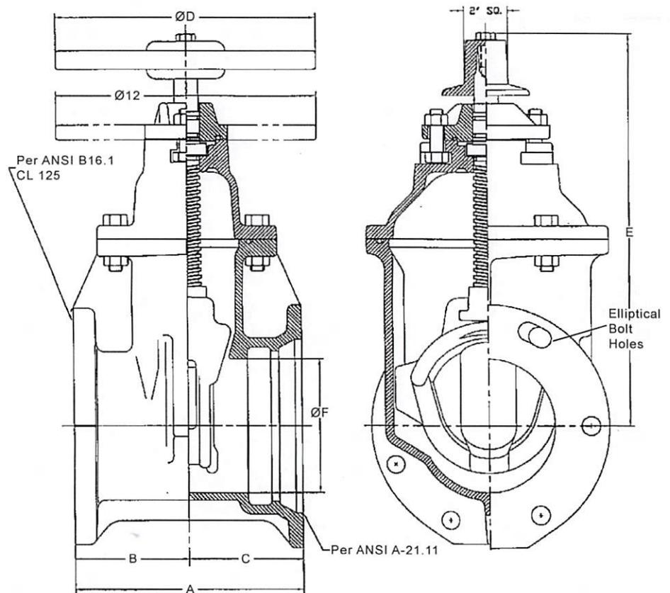
Elliptical bolt hole design eliminates the needs for anti-rotational bolts.
